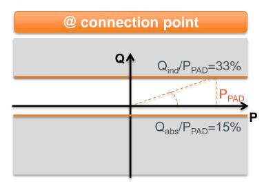
Transformer Q losses included in load @ connection point
